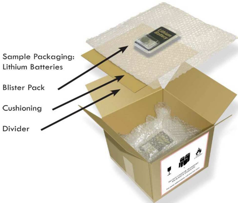
FIGURE 2. Lithium Battery Packaging Example [1].
